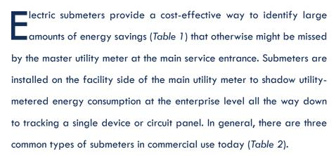
The first two types—feed-through and current transformer (CT)-based—are socket meters. CT-type socket meters typically are used with loads of 400A and above. In commercial applications, the extra space required for CT cabinets and meter bases diminishes available rental space. Additionally, socket-type meters are not UL listed. The third type is the solid-state electronic submeter, a non-socket device that provides several operational advantages, including space savings.<sup>1</sup>
